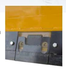
Designed for easy field service, each section of cutting edge uses 2B2N maintenance. This simple 2 Bolt - 2 Nut design makes maintaining each 12" section an easy one person job. Removing the hardware, which holds the retaining plate in place, allows for easy access to the individual components for that section.
